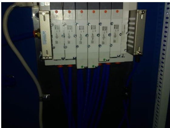
Left: Bottom of air valves with all lines. Right: Air valves.
