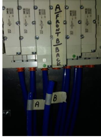
Left: Valve block assembly, as connected. Right: Lines need to be reconnect to bottom of valve block.
