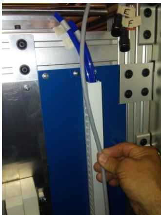
Grey cable goes into white track (near E&F).
