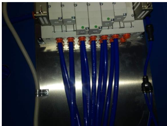
Valve block assembly as, connected. Right: Air lines regulator .
