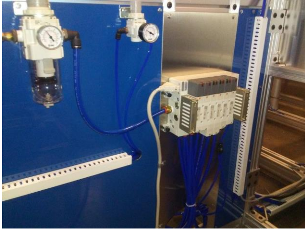
Left: Valve block assembly, as connected. Right: Lines need to be reconnect to bottom of valve block.
