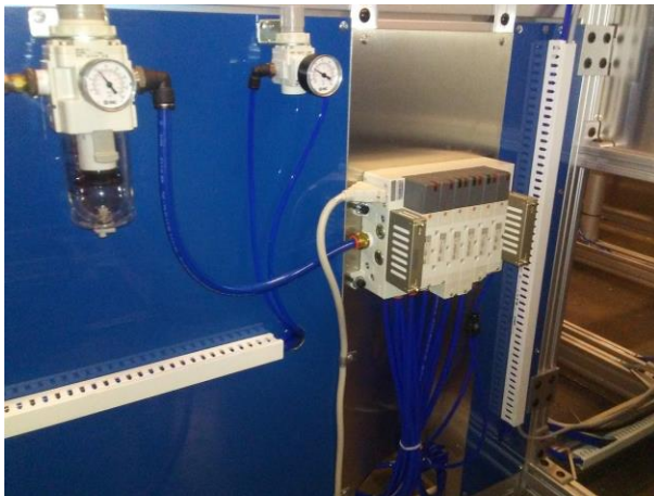
Valve block assembly as, connected. Right: Air lines regulator .
