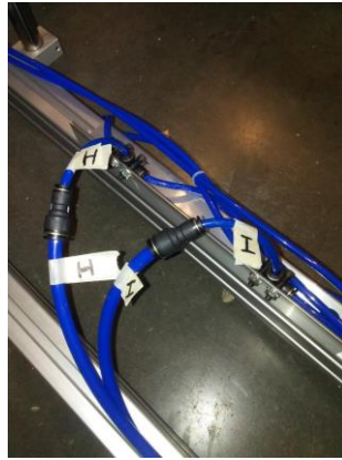
BLUE Air lines to air blocks. A few need to be reconnected, with black connector, Like "H" & "I", on right.
